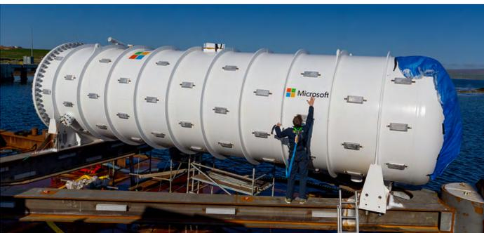
**Fig 2:** Microsoft's Project Natick, already in advanced field trials, puts an entire data farm in a submersible cylindrical container 12.2 m long and 2.8 m in diameter, using sea water as its substantial heat sink and operated from a remote location. (Image source: Microsoft)
